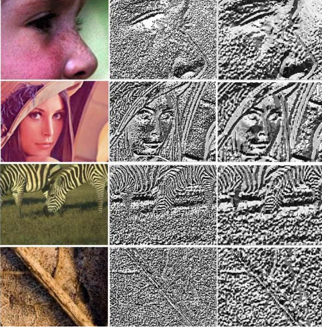
Fig. 7. Illustration of LBP maps. The left column shows some HRIs; the middle column shows the LBP maps of the HRIs; the right column shows the LBP maps of the bicubic upsampled images.
