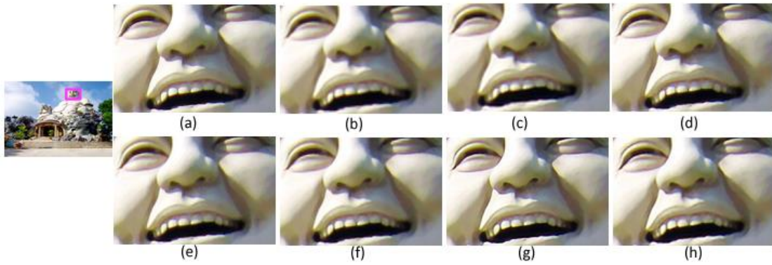
Fig.S-6. The 1.5 \times upsampled results with different methods. (a) the HR images, (b) bicubic, (c) ANR [13], (d) LPE [16], (e) SRCNN [17], (f) VDSR [18], (g) ResNet, (h) the proposed FAST.
